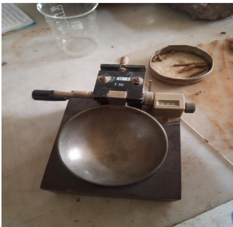
Figure 3: Apparatus used in the Liquid Limit Test
